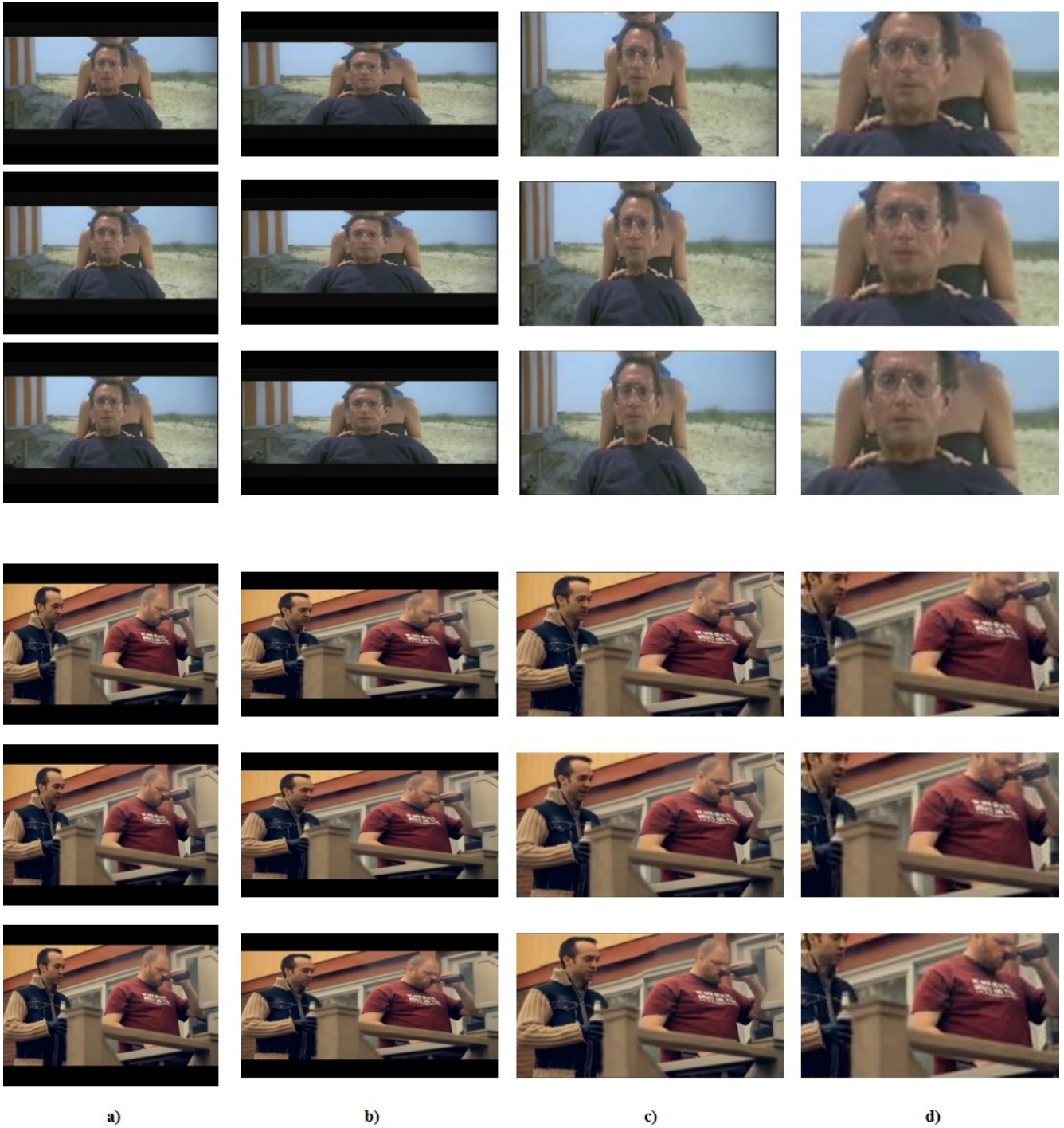
Figure 4: a) The original frames. b) Results of linear scaling. c) Results of seam carving (Yan et al., 2013) d) Results of proposed crop based retargeting. Figure best viewed in color, where problems of both approaches become obvious.
