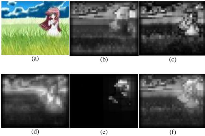
Figure 2. Example feature maps based on the concept of saliency. (f) shows the final saliency map, while (b), (c), (d) and (e) show the conspicuity maps for colour, intensity, orientation and skin, respectively.
