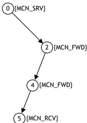
Fig. 3. The virtual tunnel approach to bandwidth availability.  $n_0$  checks for two times QoS bandwidth since it has to make sure that  $n_2$  can also forward packets.  $n_2$  checks for three times QoS bandwidth since, in addition to its predecessor  $n_0$  and itself, it has to make sure that  $n_4$  can also forward the streaming data. Finally,  $n_4$  checks again for two times QoS bandwidth since  $n_5$  is only a receiver which does not send packets.
