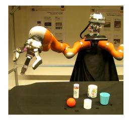
Fig. 3. The robot arm and gripper are used for manipulation, and Kinect is used to compute object features. Several objects are included while learning and verifying the planning capability in the real world.
