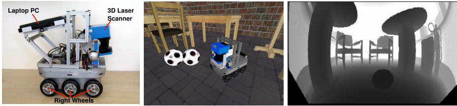
Figure 1: Left: The KURT3D mobile robot platform. Center: KURT3D simulated in MACSim. Right: A 3D range image obtained from the KURT3D.
