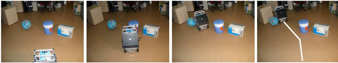
Fig. 8. The initial position of the robot is shown in the left-most figure. The robot first goes forward, then turns left since trash-bin does not afford traversability. Third snapshot shows the robot driving over the spherical object. The path of the robot is shown in the last figure.
