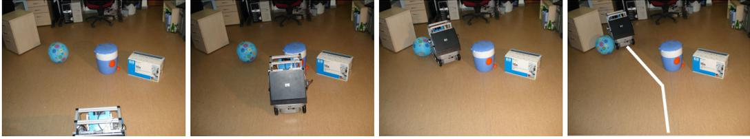
Figure 6.8: The course of the real robot trained with curiosity-driven scheme. The initial position of the robot is shown in the left-most figure. The robot first goes forward, then turns left since trash-bin does not afford traversability. Third snapshot shows the robot driving over the spherical object. The path of the robot is shown in the last figure.
