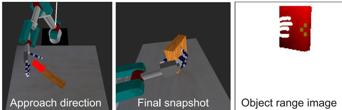
Figure 9.2: The execution of power-grasp behavior and the final object range image. The arrow shows the corresponding approach direction ( $\alpha$ ).
