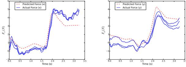
Fig. 4: Forces for robot execution with tactile feedback with object on its default position. Dashed lines correspond to the predicted force feedback obtained from GMR and solid lines correspond to the actual force feedbacks.
