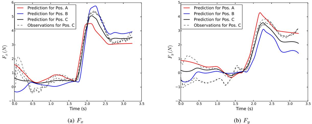
Fig. 6: Generalization of tactile feedback in (a) forces in  $x$  direction and (b) forces in  $y$  direction. Red line corresponds to forces when the wrist angle equals to 0.7 rad, Pos. A; blue line corresponds to forces when the wrist angle equals to 0.2 rad, Pos. B. Dashed lines represent forces of 3 demonstrations when the wrist angle equals to 0.45 rad, Pos. C. The green line corresponds to the GMR reproduction of these three demonstrations.
