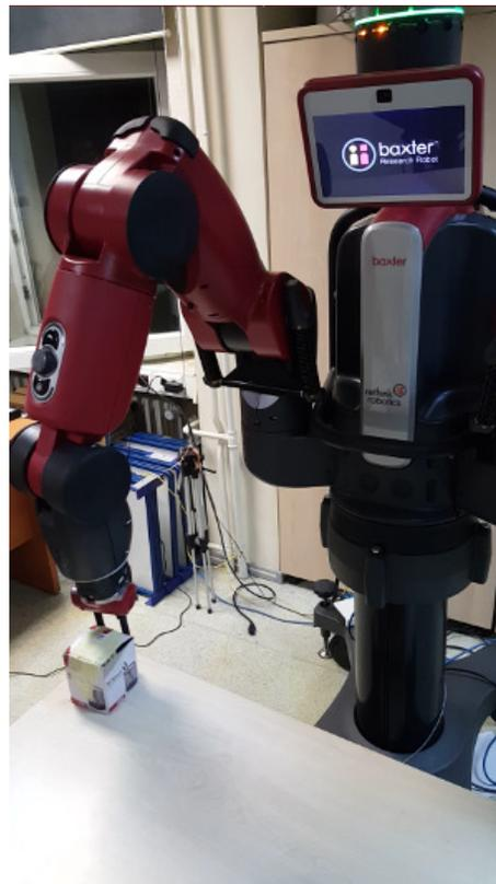
Fig. 1: Baxter robot pushing an object on table along a curved trajectory to a goal position.
