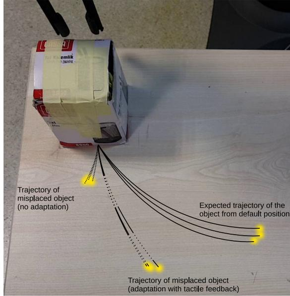
Fig. 5: The final positions of the object in different configurations, and the corresponding approximate trajectories. See link for the video : <https://youtu.be/nxdP5QiyUY4>
