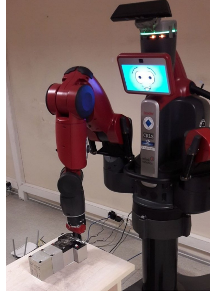
Fig. 1: Experimental setup showing Baxter robot pushing 7.5 kg battery pack.
