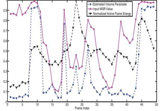
Fig. 2. Gain Estimation Problem Reasons: Low Input MSR and Low Active Frame Energy.
