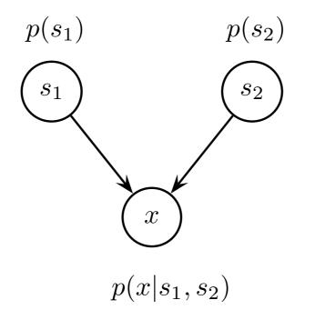
This graph encodes the joint:  $p(x, s_1, s_2) = p(x|s_1, s_2)p(s_1)p(s_2)$
