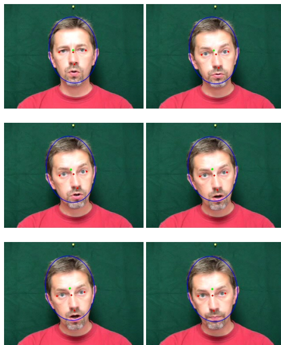
Figure 12: Results of the global head movements tracking .The ellipse and the green point are the results of last year, red points is the new tracking method.
