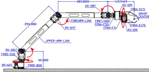
Figure 1. Mechanical design of the manipulator (Degrees of freedom shown in red, all dimensions are in mm).
