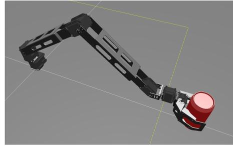
Figure 2. The simulation model of the manipulator, about to grasp a soda can.
