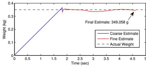
Figure 3. Example weight estimation of a 350g object.
