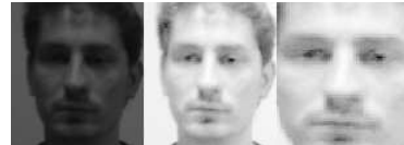
Fig. 14. a) The original captured frame. b) The illumination compensated image. c) The result of the adaptive cropping
