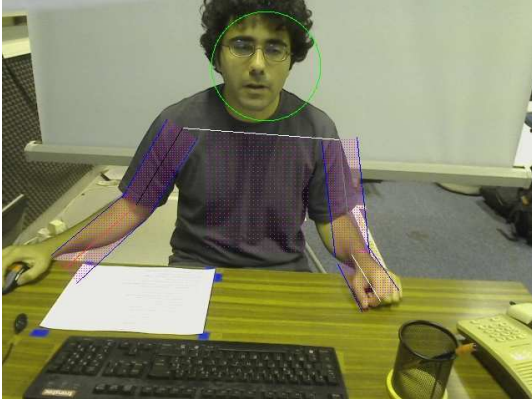
Fig. 3. Projection of the flesh model associated to a given particle
