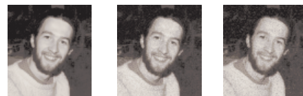
Original Gaussian Salt-and-pepper sigma=20 p=0.3 mean=0
