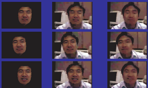
(a) The synthesized face motion (b) The reconstructed video frame with synthesized face motion (c) The reconstructed video frame using H.26L codec.
