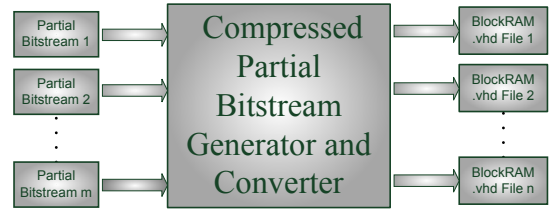
Fig. 4. File conversion from partial bitstream file to BlockRAM coefficient file
